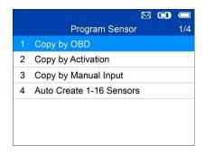
There are four ways to program MX-Sensors: Copy by OBD, Copy by Activation, Copy by Manual Input and Auto Create 1-16 Sensors.
