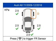
All sensors have been triggered. Display advances to Sensor Status screen even if not all sensors have been successful activated.
