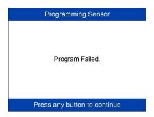
A failure message will display if the sensor fails to program. Press any button to continue. Ensure you are using an MX-Sensor are that you are using the correct frequency. Try to program sensor again.
