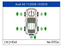
If no DTC are present in the ECU, the middle TPMS icon displays gray and a "No DTCs" message displays at the right bottom of the screen.
