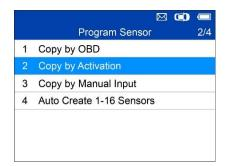
Select Copy by Activation from programming list. Activate or Trigger sensor to be copied.
