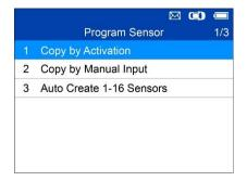
Press Y to select Copy by Activation. Place the tool near the sensor to be copied. If the sensor is still attached to the wheel, hold the close to the tire sidewall right above the sensor.
