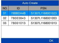
Once the sensors are successfully programmed, the sensor IDs and the PSNs will display on the tool.
