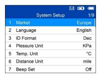
Figure 5-9 Sample System Setup Screen
