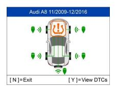
Use Up and Down Arrow button to select the TPMS icon in center of graphed vehicle and press **Y** to view the DTCs.
