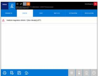
The Errors page instantly displays all the **errors in the vehicle**, with the related codes and descriptions. From this page, the error **reading** and **clearing** can be carried out in a single click, as well as a **self-diagnosis test** on the selected system.
