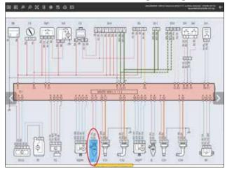
The **animations of the relevant devices** create an interactive map with the flow of input and output signals to/from the control units.
