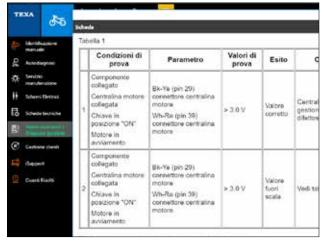
Useful to solve a **fault associated with an error code** detected in self-diagnosis. They provide a tree diagram to solve the fault
