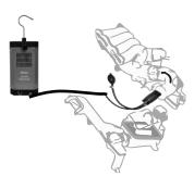
5. Connect Power Cords to 12V vehicle battery. For best performance, the vehicle battery shall be fully charged. Do NOT use a DC12V switch power supply.
