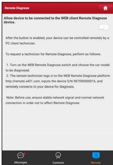
1. Slide the switch “Allow device to be connected to the WEB client remote diagnostic device” to ON so that the partner can find and connect to this device while using the PC.
