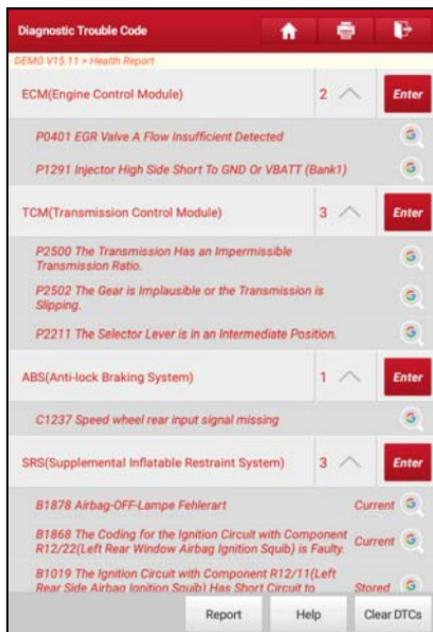
The tested system with fault code appears in red and the system with OK displays in black (normally).
