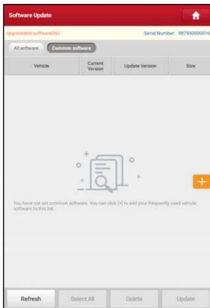
Tap “+” on the right edge of the screen, a pop-up window appears. Select the checkbox before the software name and tap “SAVE”, the software will be displayed in the Common software list. Next time you want to update it, just go to “Common Software”.
