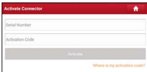
Input the Serial Number and Activation Code, and then tap “Activate” to activate the connector.
