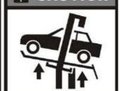
Auxiliary adapters may reduce load capacity
