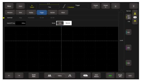
**Common** allows you to set the sweep mode. The sweep mode determines how the Scopebox behaves in the absence of a trigger event. The Scopebox provides two trigger modes: Auto, Normal.
