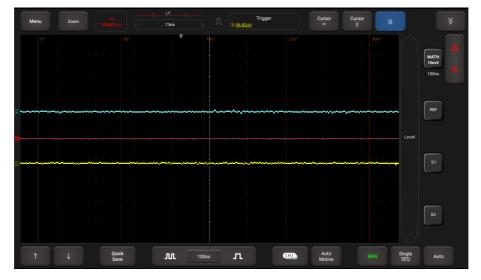
You can drag the two phase rulers to the appropriate position to mark the start and end of the loop. The bottom of the ruler shows the default phase start point 0° and end point 360°, which can be edited to any value. For example, when measuring the timing of a four-stroke cylinder, the end of the phase is usually displayed as 720°, because one cycle includes two crankshaft rotations.
