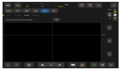
Tap **OK** on the pop-up message box to start calibration. The LED on the Scopebox starts flashing and the prompt message "Self Adjust is running" will appear on the upper left corner of the screen.
