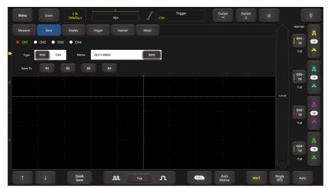
Select the desired measurement channel and save type (.WAV or .CSV), tap the default file name to revise it. Tap **Save** to save it. Alternatively, the user can save the waveform files to the designated folder (R1, R2, R3 and R4). If the files are saved under the folder, the user can recall the saved files (go to **Userset -> Save Recovery**) for reference and play back.
