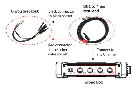
4. Connect the black terminal and signal wire (its other end connected to the red 4mm connector) of the 6-way breakout lead to the GND and signal terminal of the vehicle sensor.
