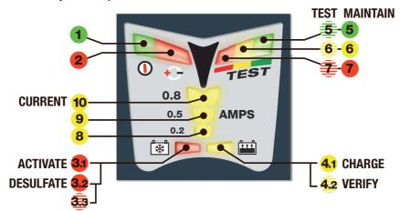
1. LED #1 - Power on. This LED confirms AC power supply to the charger.
