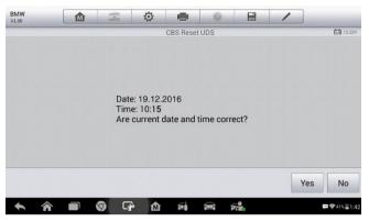
Figure 7-2 Sample Oil Reset Service Screen 1
