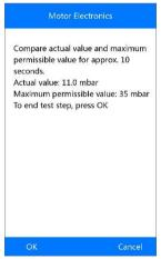
Figure 5-41 Sample Exhaust Backpressure at Idle
