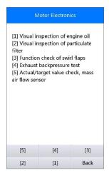
Figure 5-32 Sample Particle Filter Tests
