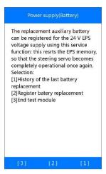
Figure 5-65 Sample Auxiliary Battery Functions
