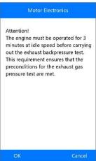
Figure 5-39 Sample Exhaust Backpressure Test Attention
