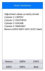
Figure 5-25 Sample Injection Rate Adjustment Screen
