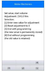
Figure 5-21 Sample Starting Basic Inspection Quantity Functions
