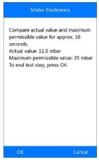
Figure 5-42 Sample Exhaust Backpressure at 2000 RPM
