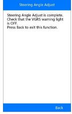
Figure 5-12 Sample Steering Angle Adjust Completed Screen
