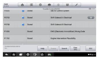
Figure 4-19 Sample DTC & FFD Screen
